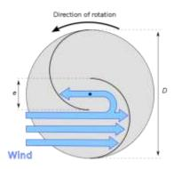
Fig. 6: Working of a Savonius turbine (Source: By Ugo14 - Own work, CC BY-SA 3.0)
