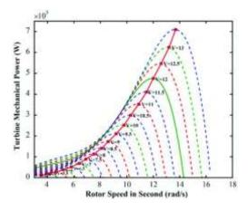
Fig. 7: Turbine mechanical power curve vs. rotor speed under variable wind speeds as seen in Sarkar et al. [32]
