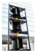
Fig. 5: Darrieus Wind Turbine (Source: Wikimedia Commons)
