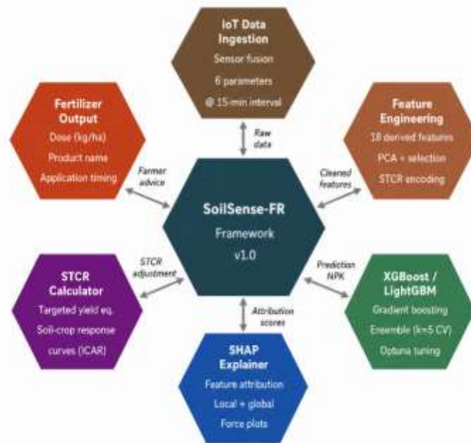
Figure 4. SoilSense-FR Architecture with XGBoost, LightGBM, SHAP, and STCR Modules [18], [19], [21], [22]
