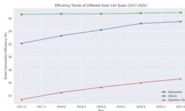
Figure 2: Efficiency Trends of different solar cell types
