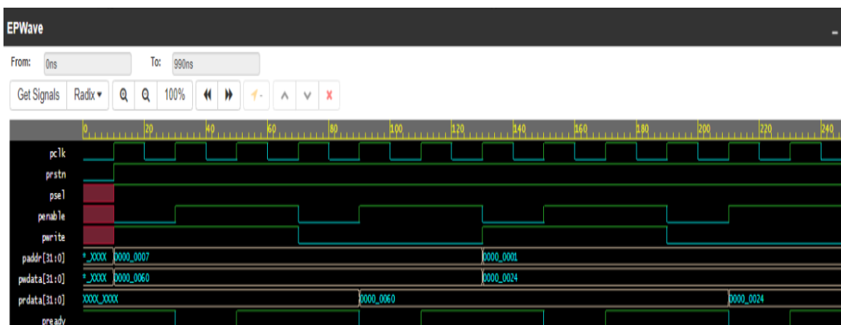
Fig 7: APB Read Transfer with Wait States
