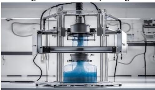
Another clear difference between solution electrospinning and melt electrospinning lies in the handling of the polymer medium. Unlike solution electrospinning, where a fluid line can be
