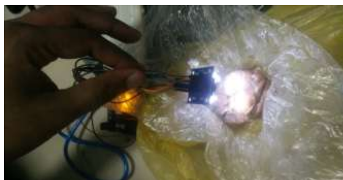
Fig. 12. Color sensor measuring meat freshness
