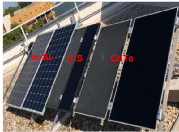
Fig. 3 shows the setup done on University of Jaen's rooftop for researchers in [15].
