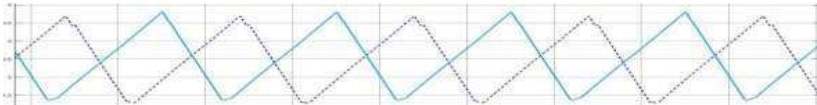
Fig. 14(a) The current of inductors L1 ( i_{l1} ) and L2 ( i_{l2} ), i_{l1} = 3.6 A, i_{l2} = 3.8 A
