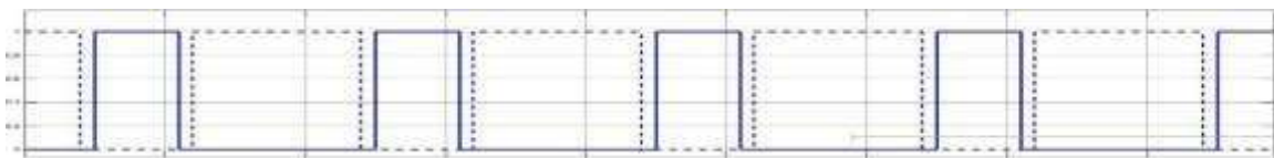
Fig. 11 Gate pulse for Switch S1 and S2 for 0.3 duty ratio
