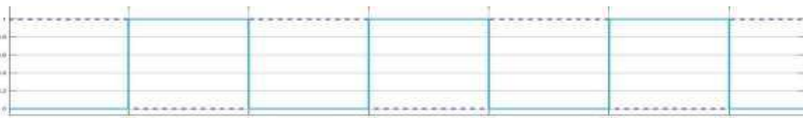
Fig. 13 Gate pulse for Switch ST1 and ST2 for 0.5 duty ratio
