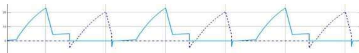
Fig. 14(e) The current through the switches S_1 and S_2 i_{s1} = 22 A, i_{s2} = 20 A
