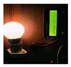
The level of voltage is 235v and the frequency is 47 Hz, those are at synchronization condition, so that the load is ON and the buzzer is OFF.
