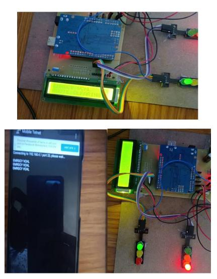
When the input receives the supply. The LCD will be switched on with the project's name shown in the window. And now the machine is functioning well. This diagram illustrates how the project's title will appear on an LCD screen. And the functioning of the traffic signals will be shown.
