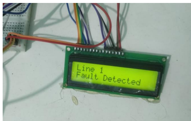
Fig 5.4: Line 1 Fault Detection- LCD Notification
