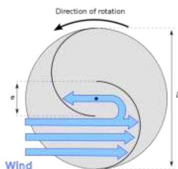
Fig. 6: Working of a Savonius turbine
