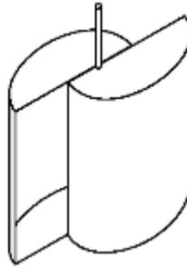
Fig. 7: Schematic drawing of a basic Savonius turbine
