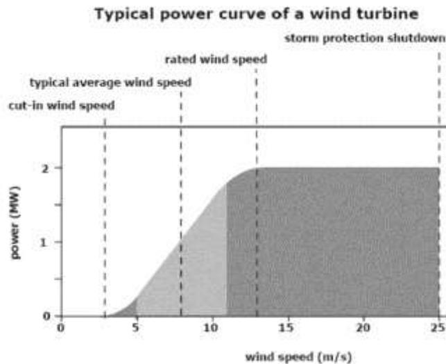
Fig. 3: Typical Power Curve of a Wind Turbine [7]
