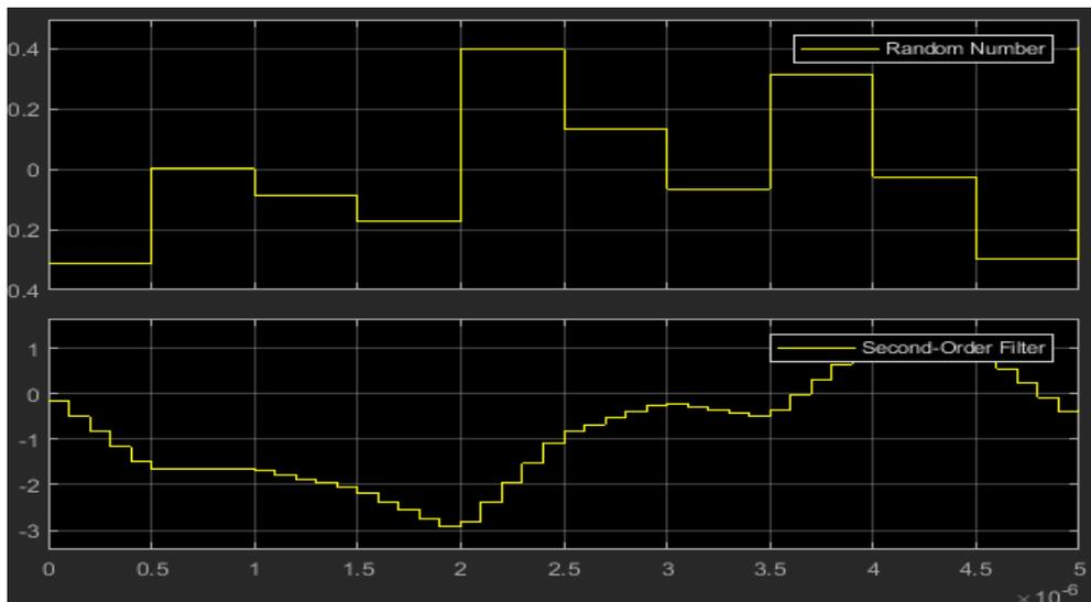
Figure 9: The achieved analog message signal from the signal generator.
