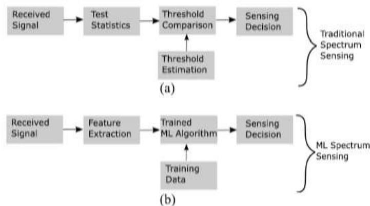
Figure 4: Spectral sensing methodology (a) Applying the conventional method and (b) Employing ML-based methods [10-18].
