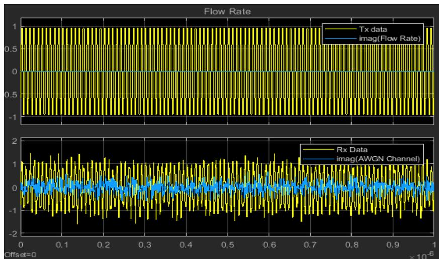
Figure 13: The obtained corrupted OFDM signal after passing through the AWGN channel.
