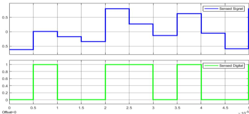
Figure 10: The message signal in both analog and digital form before and after the ADC system.
