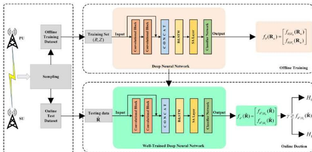
Figure 1: Typical 5G LTE spectral sensing deep learning technique block diagram [3-6].
