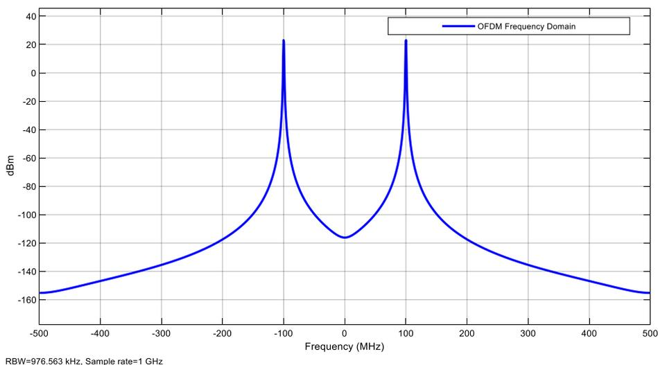
Figure 12: The spectrum of the OFDM modulated signal is obtained by performing Fourier transform with  $f_c=100$  MHz.
