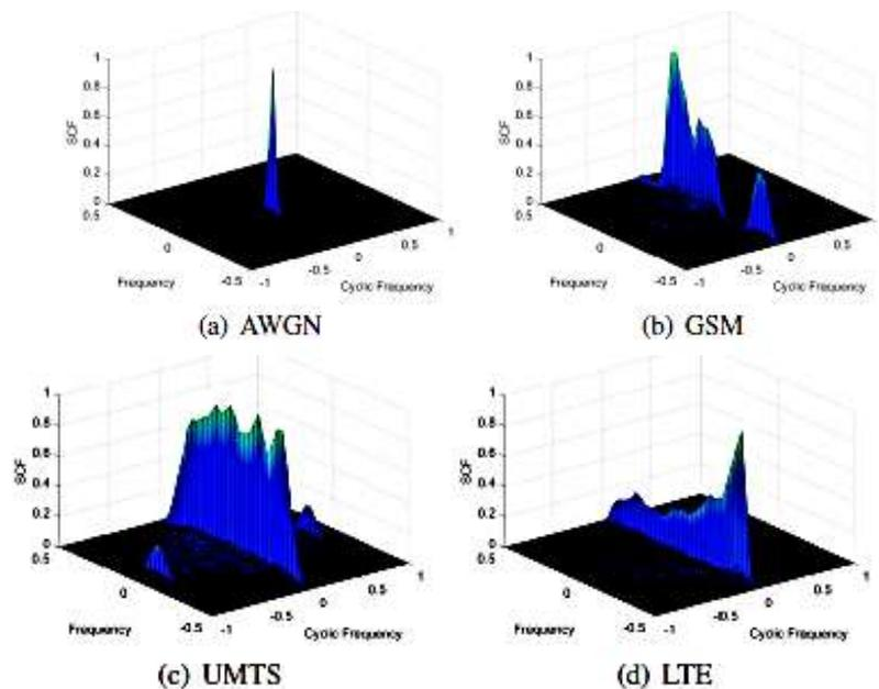
Figure 2: Estimations of cellular waves in the bi-frequency surface made by PSD using FAM. The various cyclic characteristics of the signals might be simply observed. Since the noise's PSD just yields a amplitude at the middle of the bi-frequency surface, where the cyclic frequency is zero, the noise exhibits no cyclic characteristics [10-14].
