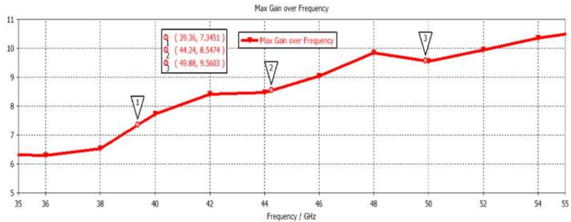
Fig. 14. Simulated max gain over frequency for the proposed PRGW antenna
