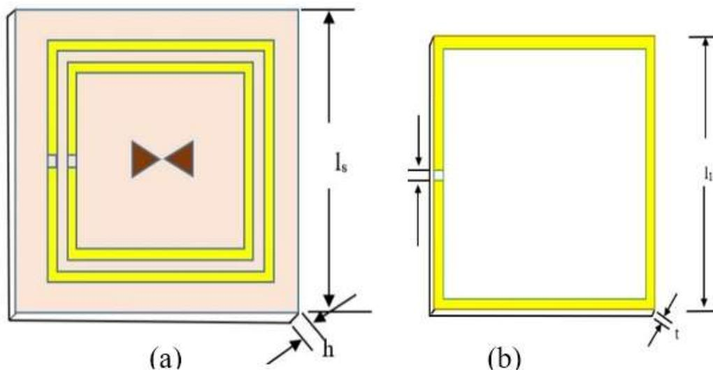
Fig. 7. (a) Optimized design of the PRGW antenna, (b) Optimized design of Unit Cell design
