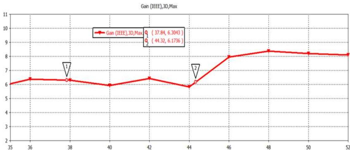
Fig. 10: Gain curve for dual-band PRGW antenna
