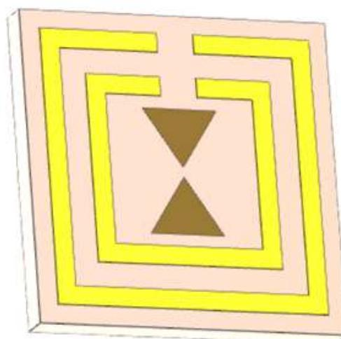
Fig. 04. PRGW Antenna with bow-tie slot
