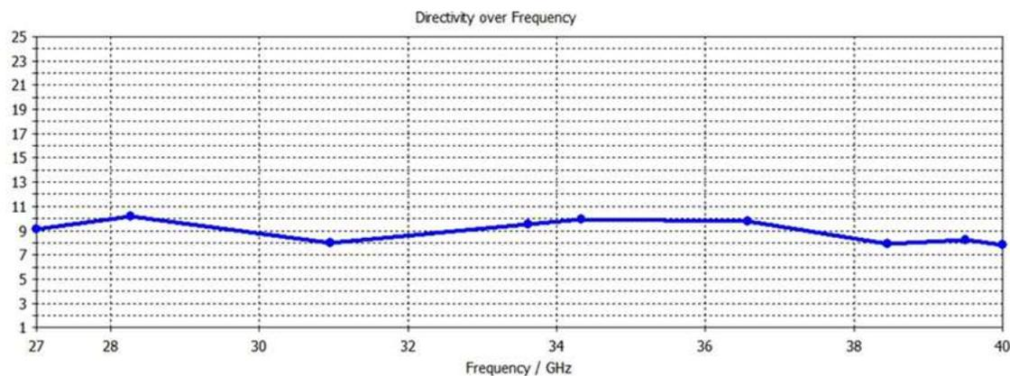
Fig. 15. Simulated directivity over frequency for the proposed PRGW antenna
