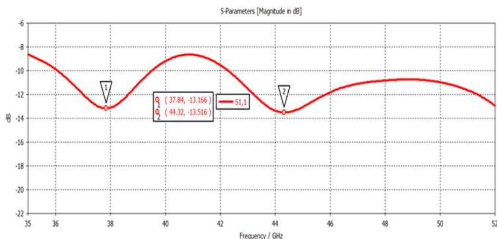
Fig. 8. Simulated S11 or Return loss dual-band for PRGW antenna.
