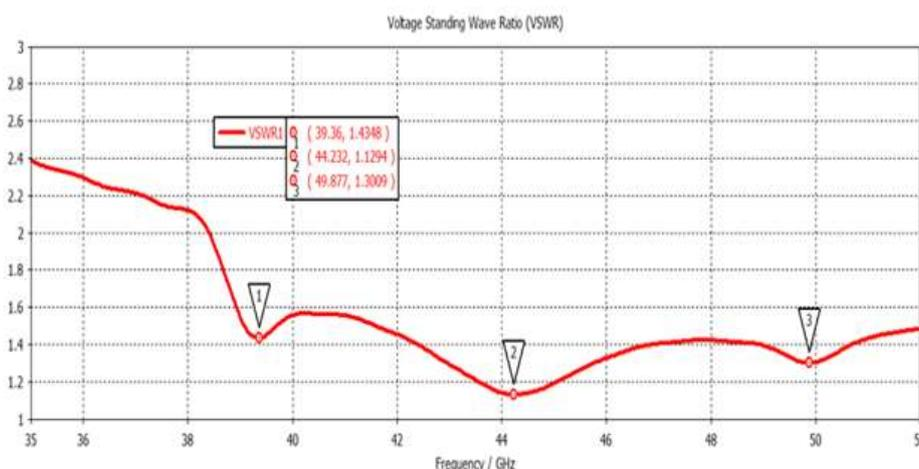
Fig. 13: VSWR curve for triple-band PRGW antenna
