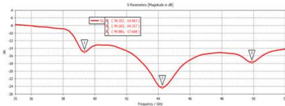
Fig. 12: Simulated S11 or Return loss triple-band for PRGW antenna
