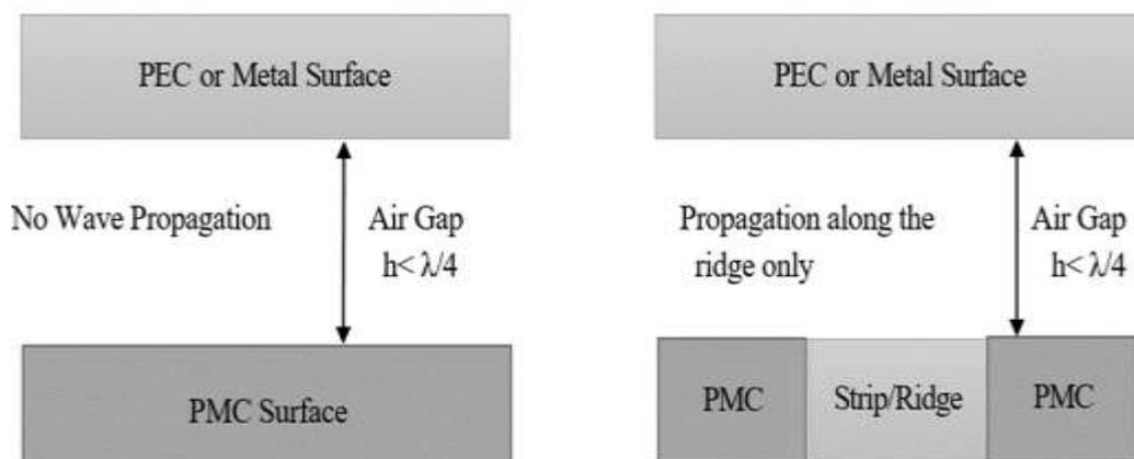
Fig. 01. (a) Parallel plate of PEC and PMC with air-gap, (b) Surface of PEC/PMC around Ridge.
