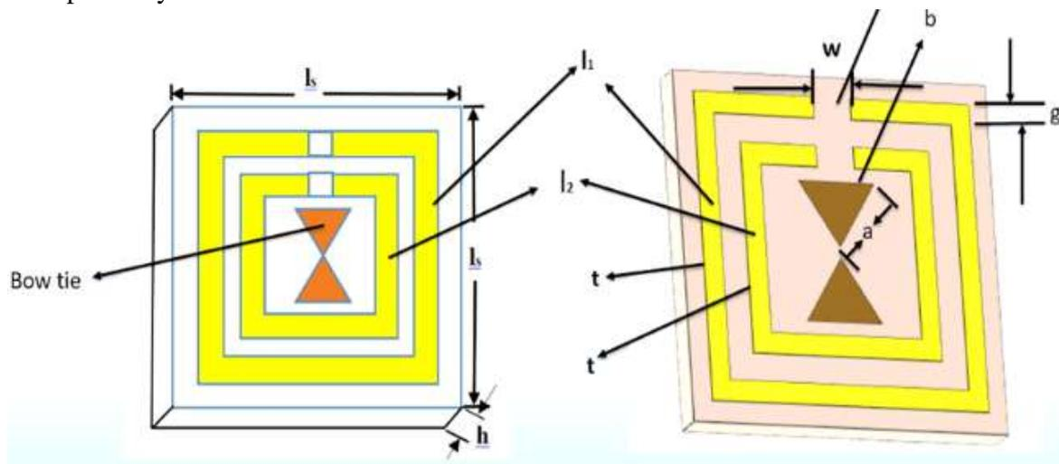
Fig. 05. PRGW Antenna with bow-tie slot with parameters
