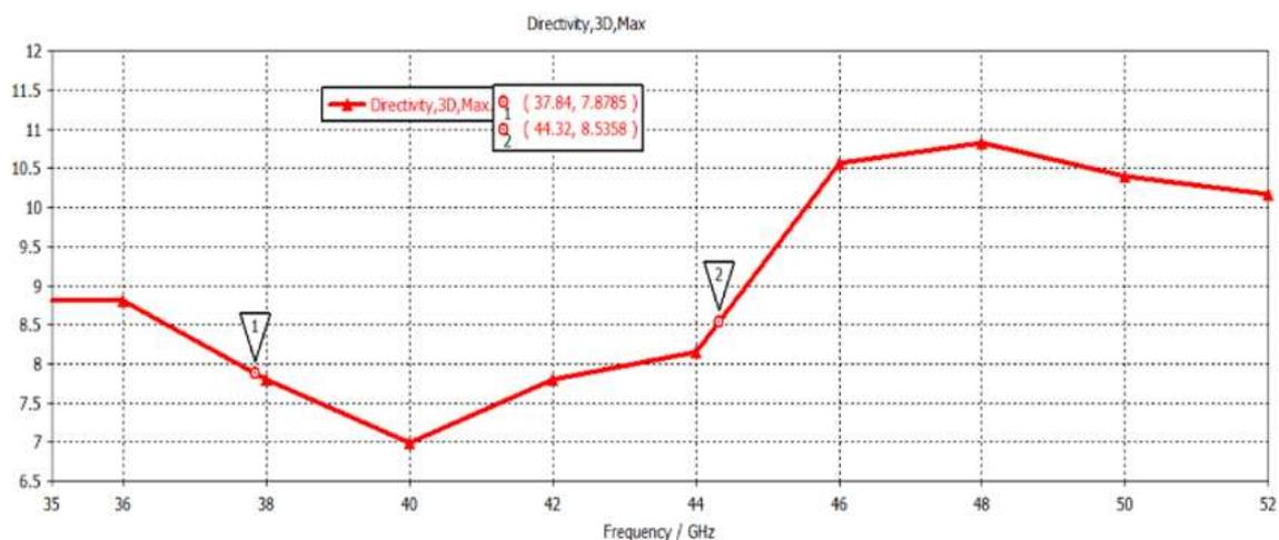
Fig. 11: Directivity curve for dual-band PRGW antenna
