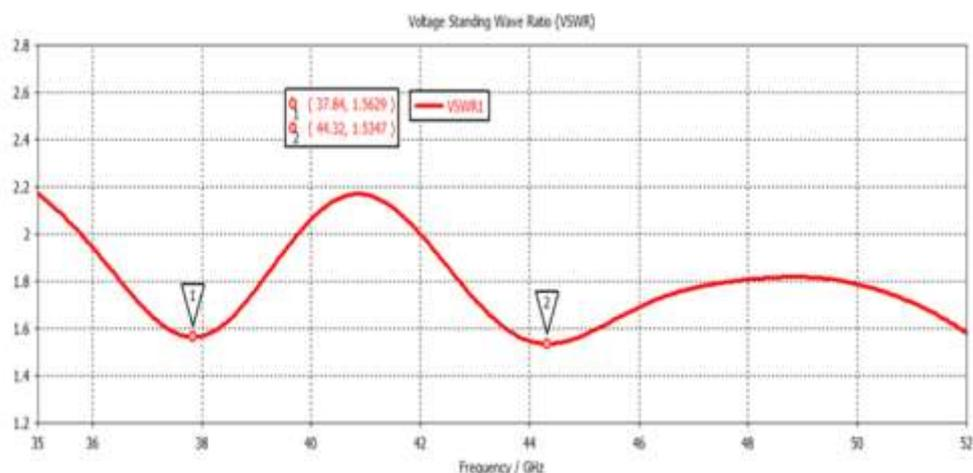
Fig. 9: VSWR curve dual-band for PRGW antenna Dual-band antenna at resonance frequencies  $fr_1$  and  $fr_2$  are gain and directivity shown in "fig. 10" & "fig. 11".
