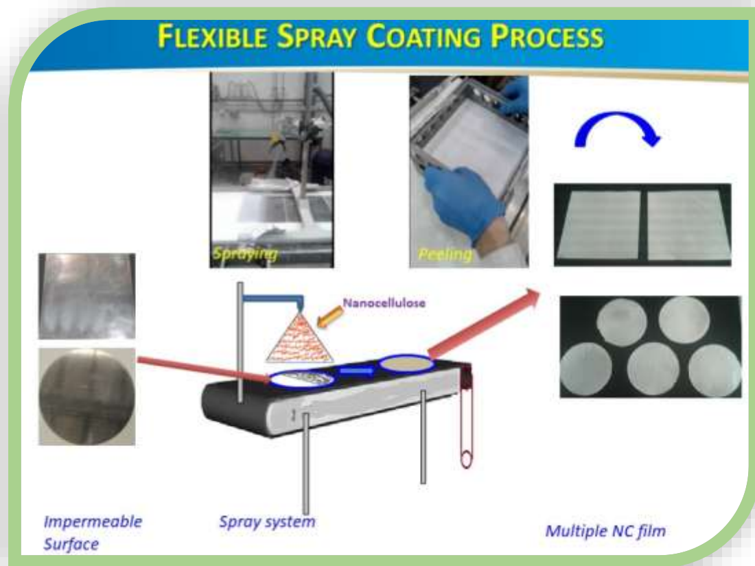
Figure 7 – An experimental set up for spraying CNF suspension on the stainless steel plate
