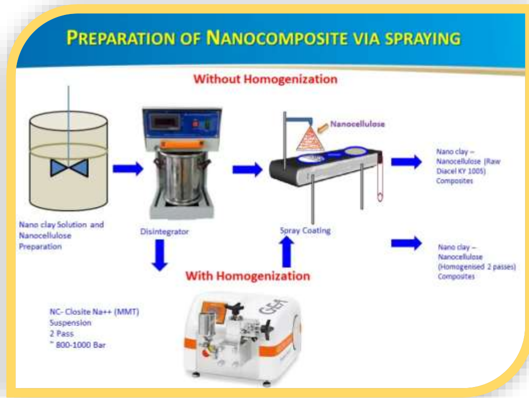
Figure 8 – An experimental set up for spraying CNF -MMT suspension on the stainless steel plate.
