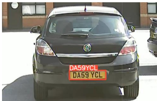
Fig.12: Model successfully detecting and Reading Number License Plate. Source: Frame from a YouTube Video [18]
