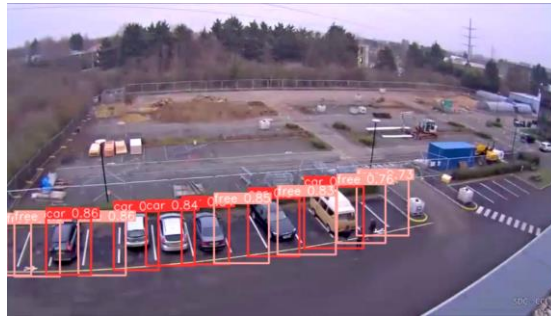
Fig.10: Model successfully detecting empty and occupied Spaces. Source: Frame from Google Colab Dataset
