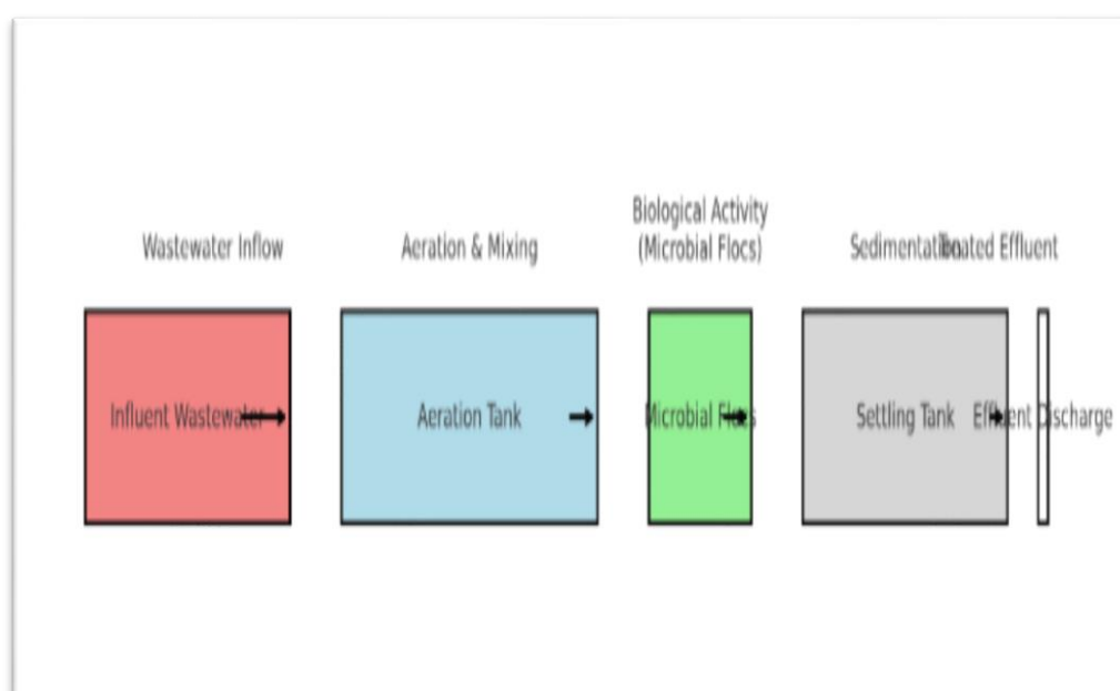
Figure 2. Diagram of Biological Wastewater Treatment Process
