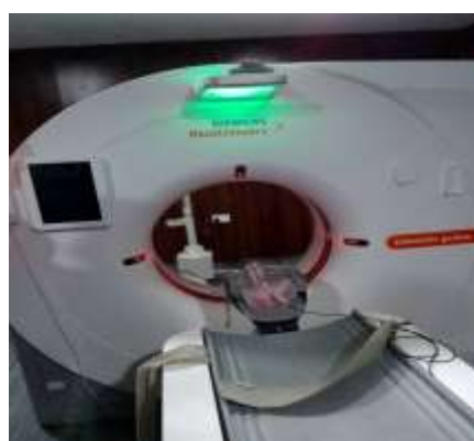
Figure 3. Standard Head Phantom with a Pencil Ionization Chamber and Insert on a CT Machine.
