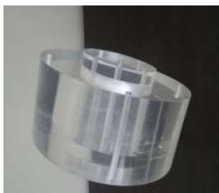
Figure 2. Standard Head and Body PMMA Phantom. [21]
