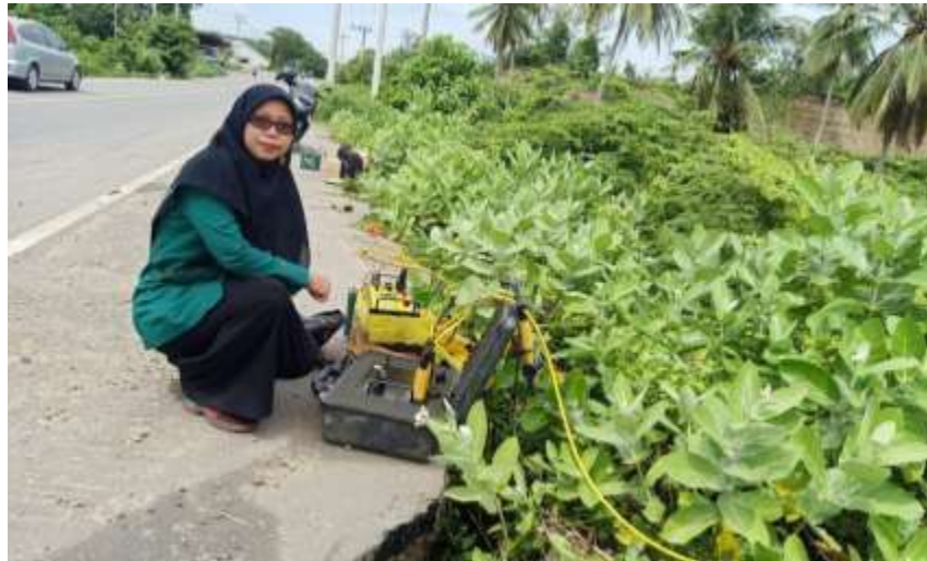
Figure 4 Measurement Process Using Resistivitymeter On ELAK1
